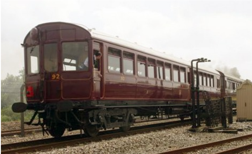
STEAM RAILMOTOR DRIVING TRAILER. NOTE ALSO THE APPARATUS FOR COLLECTING AND DROPPING OFF MAILBAGS WHILST ON THE MOVE.
