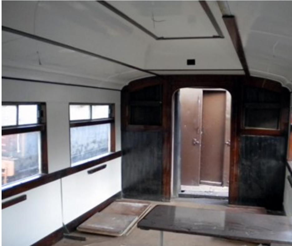
New ceilings and wall panels with the restored trim being replaced
