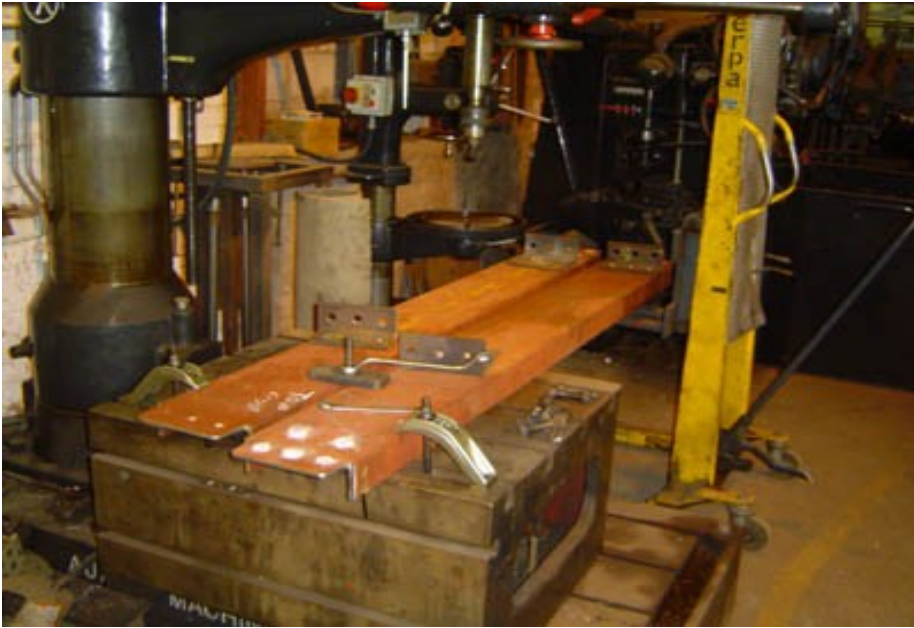
Cutting out the bent longitudinals and the new ones on the drill
