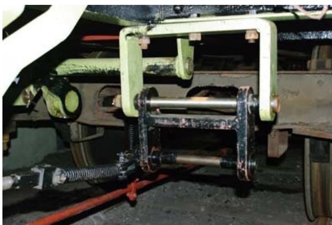
Above. Dynamo bracket in place.
